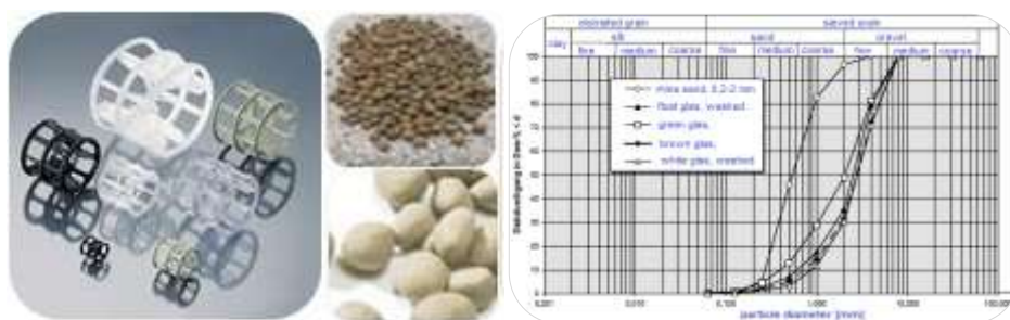
Figure 4: Moved Bed Material for MB- Reactor, ( RAUSCHERT, 1,0 kg/dm 3 , left side, from polymer), Bloated clay and- Glass (middle) and Bloated Recycling Glass sieving line (right side, below)
