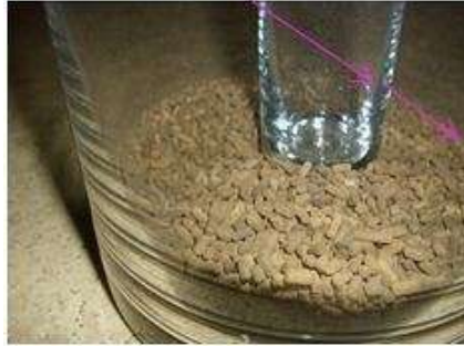
Figure 13: Reactor with external cylinder for Granules and Laser Beam (red)
