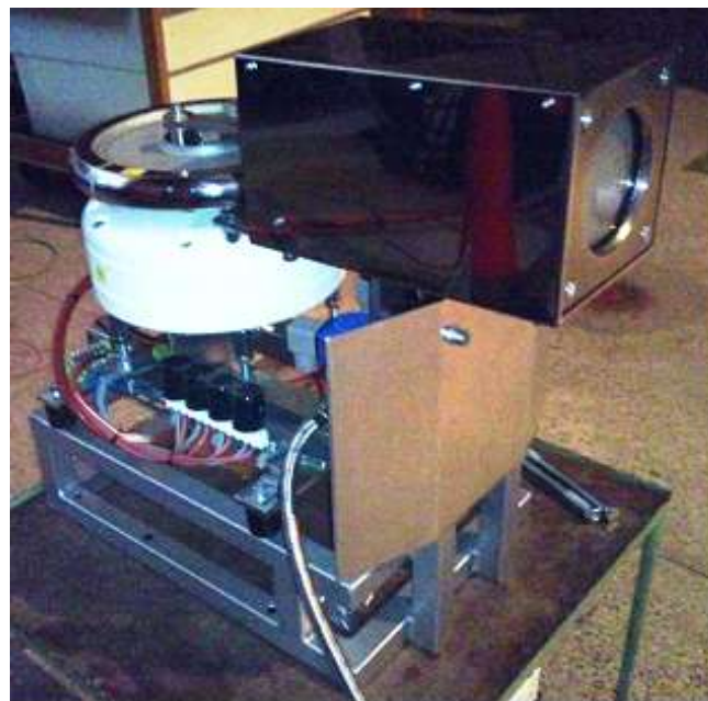
Fig.2 Block of expansion machine with electric generator
