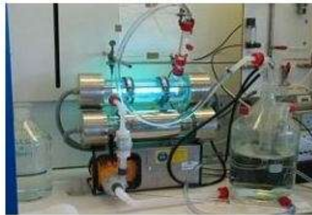
Figure 1: Photocatalytic Oxidation based on UV- Light
