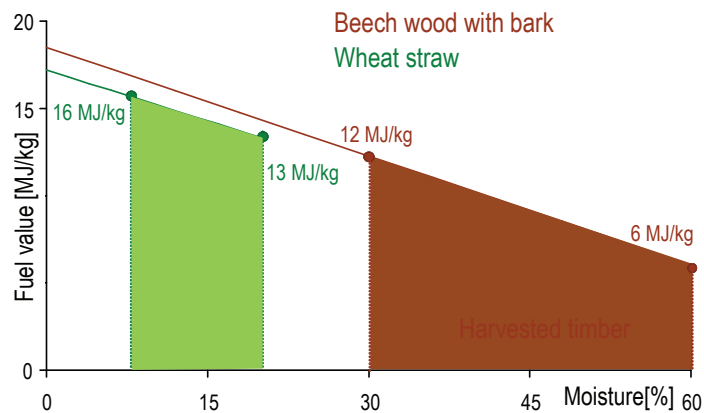
Fig. 2 Fuel moisture influence on the biomass calorific value
